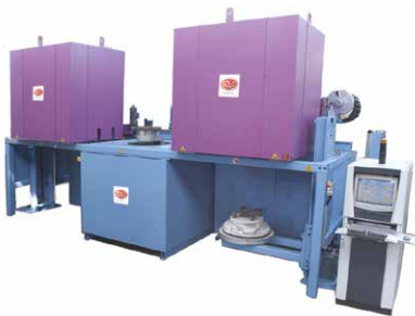
Additional quench furnace fully equipped
